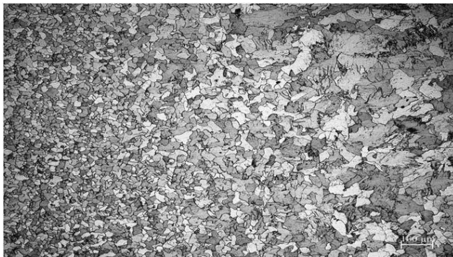
Microstructure of sample at I_m=130\text{ A} and S=0.75\text{ cm/sec}
