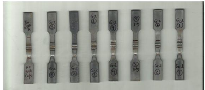
Schematic representation of the Failure of base metal during axial tensile testing of welds
